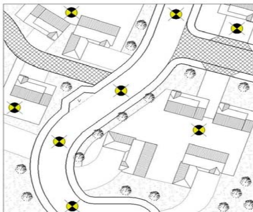
Figure 5.1 - Exploratory Borehole Survey
